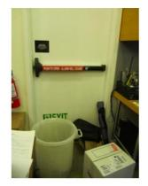
Blocked emergency equipment and blocked emergency exit.
